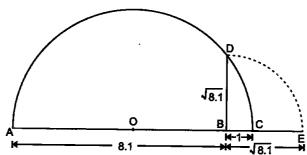
Mark the distance 8.1 units from a fixed point A on a given line to obtain a point B such that AB = 8.1 units. From B, mark a distance of 1 unit and mark the new point as C. Find the mid-point of AC and mark that point as O. Draw a semicircle with centre O and radius OC. Draw a line perpendicular to AC passing through B and intersecting the semicircle at D. Then,  $BD = \sqrt{8.1}$ .
